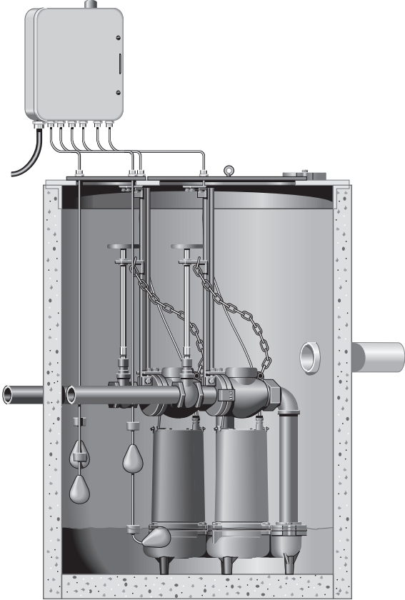
Typical Duplex Installation
